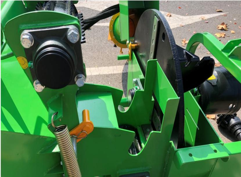
PTO shaft with friction clutch included
